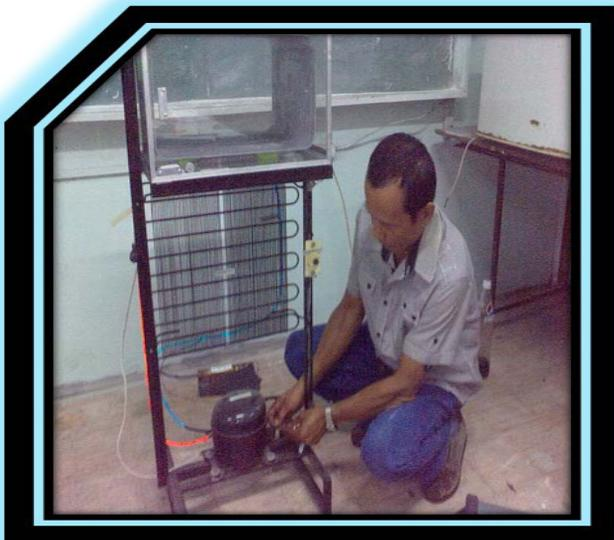
Figure 5. The developed refrigerator trainer
